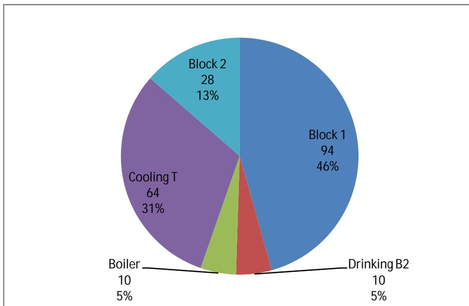
We have conducted detail HVAC system study ( Refer attached annexure) and have recommended revamping of HVAC system to suit actual requirement and save energy. These calculations have suggested that the water consumption on account of CT makeup water will reduce to 28KL from present average of 64KL per day.
