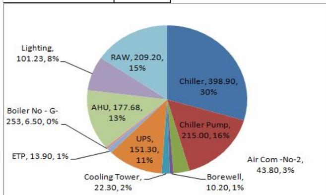
This shows that total HVAC load is 59%, which is measured and appears fixed for day time and reduces during night. The pump energy appears to be on higher side compared to energy consumption by chillers.
