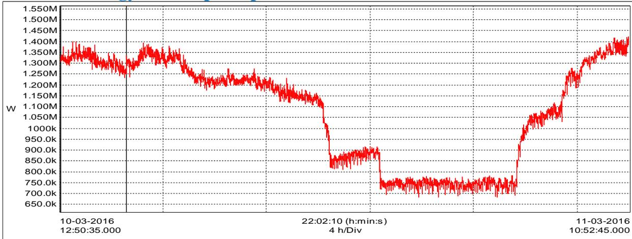
As shown above, the peak load of 1300KW prevails from 11AM to 6PM. During 1AM to 6 AM the load is around 750KW.
