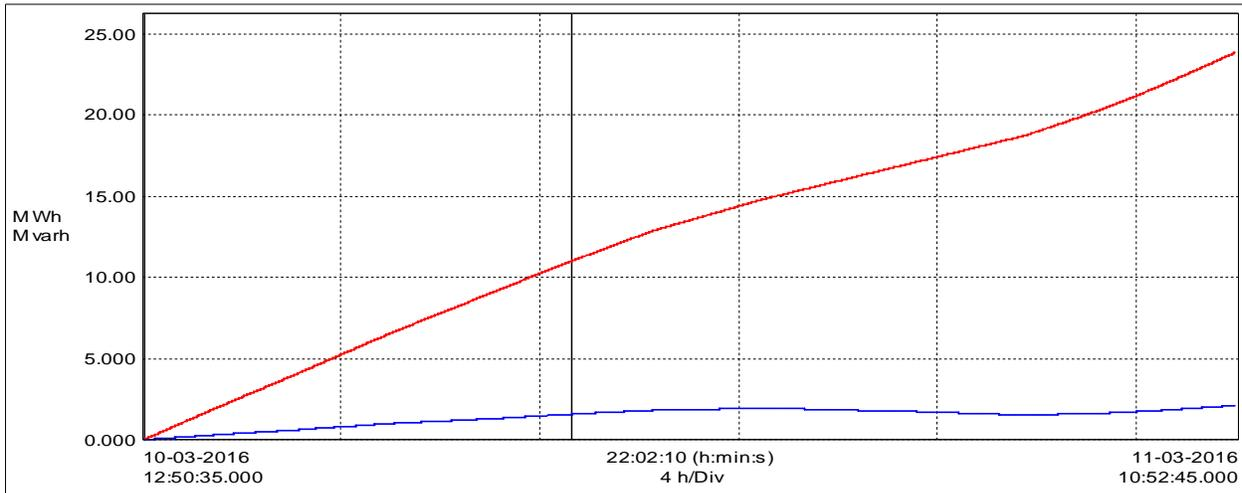
As shown above Energy consumption plot shows consumption of 23878 Kwh in 22 hours. The plot also shows continuous requirement of reactive power.
